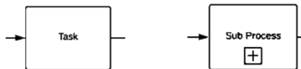
Figure 3. 3: Representation of tasks and subprocesses in BPMN
