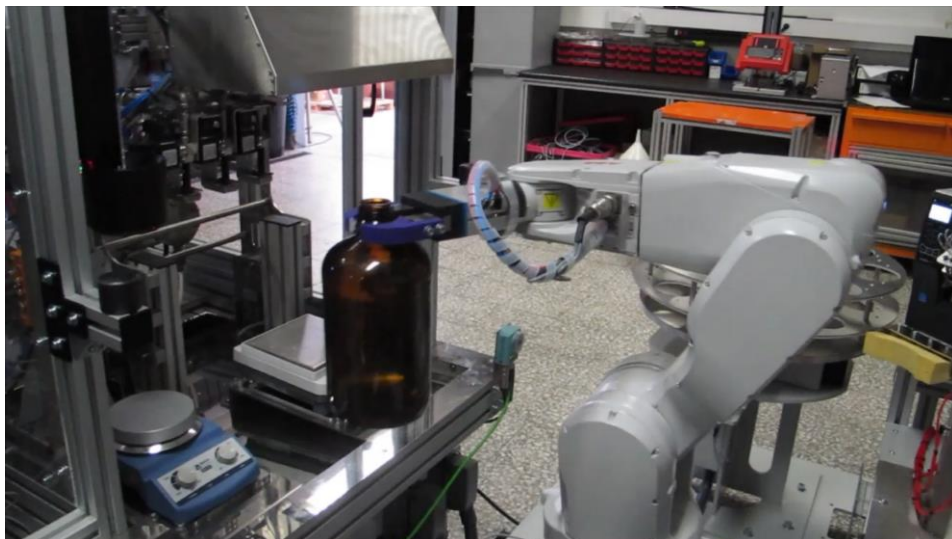
Figure 1. 5: Robot System for Solution Preparation carrying a bottle
